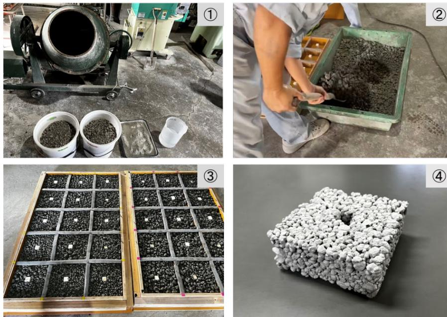
Fig. 1 Manufacturing process of block connected by drifted pumices.
