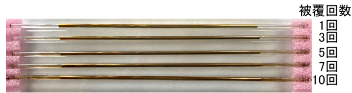
Fig. 4 Number of immersions in 5 mg/mL graphene oxide aqueous dispersion and appearance of the sensor
